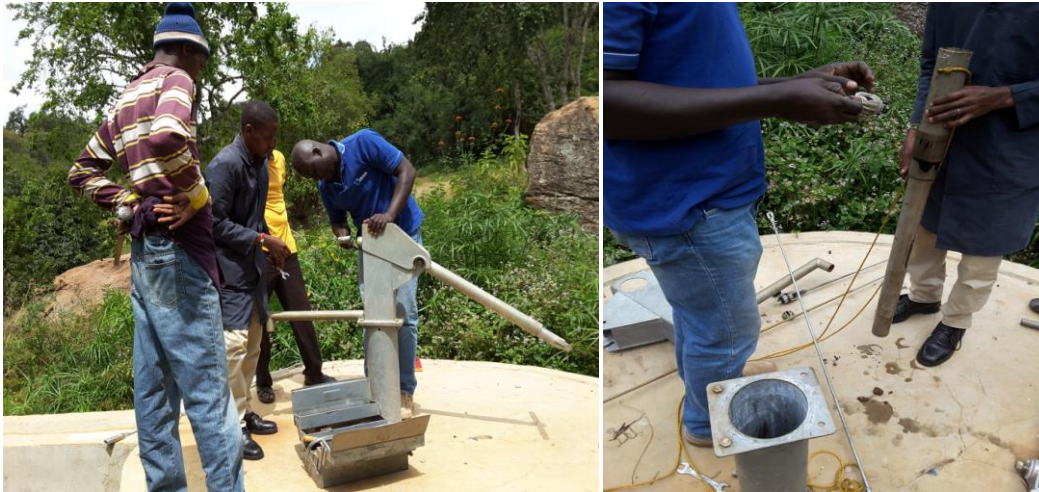
Picture above: Technical assessment of the hand pump.
